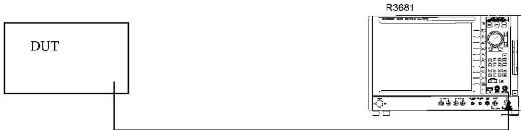
Figure 4-18 Connection Diagram for the Modulation Analysis that Uses the Multi Frame Mode
